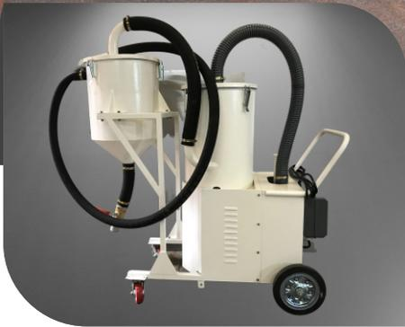
**Elektra Vac** Flux Recovery System have proven themselves as the most essential accessory to the entire Sub-Arc Welding process. They save value of flux, helps make better welds and produce all important saving in man hours. Flux Recovery unit keep abrasive flux away from moving parts on the welding ring. These systems are capable of separating out slag and fine flux returning only the clean reusable flux to the hopper.
